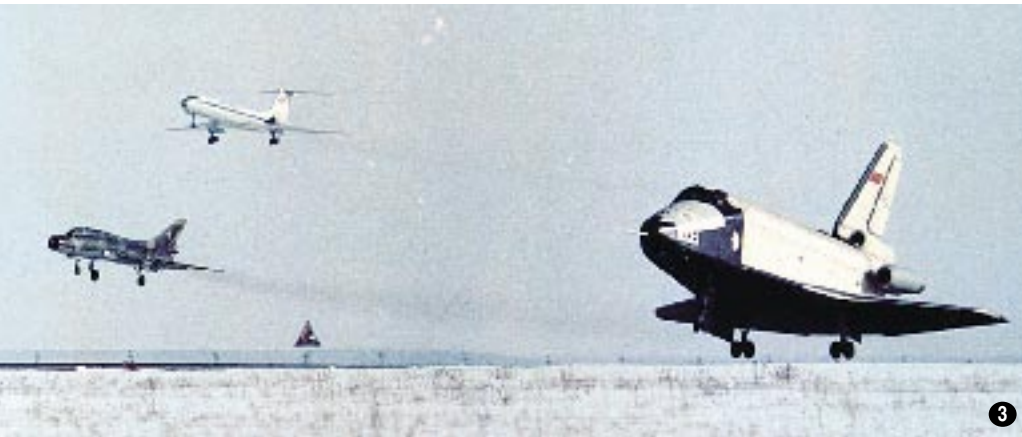
[1] Bor-2, an experimental hypersonic test vehicle, flew in December 1969 at speeds of up to Mach 13.3. A member of the family, Bor-4, achieved speeds up to Mach 25. [2] A converted Myasishchev Bison bomber carries the Buran shuttle externally, piggyback fashion. There were two such carriers at Ramenskoye. [3] A full-scale Buran replica lands after a test flight. The vehicle made several flights from Ramenskoye under its own power. Here, an Su-17 fighter-bomber (foreground) and a Tu-134 airliner fly chase.
