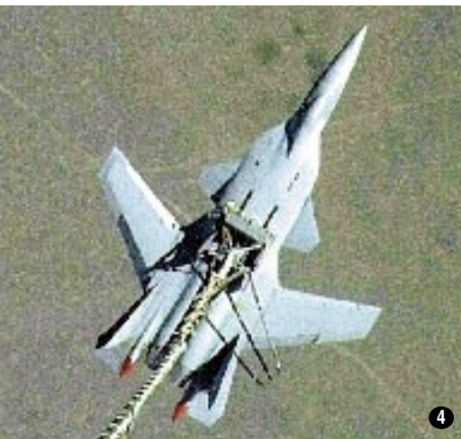
[4] A new forward-swept wing design, created by Sukhoi, is about to be dropped from a helicopter; it is a scaled-down aerodynamic test article. The full-scale aircraft, originally designated S-37 Berkut, made 61 flights in the late 1990s. [5] An Su-47 prototype fighter, shown here in a test, is said to have many advanced features. Sukhoi claims that the fighter is stealthy, having a radar cross section of 3.2 sq. ft. [6] A production Tu-144 airliner in 1995 was modified by NASA, Boeing, and Rockwell as a test bed for NASA's High-Speed Commercial Research program. Note the US and Russian flags on the tail. After 27 test flights, it was returned to storage at Ramenskoye.
