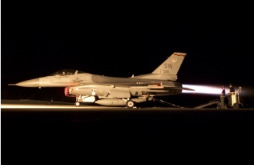
An F-16CJ runs in full afterburner during a nighttime engine test at Shaw AFB, S.C. SrA. James Kennedy controls the test from the cockpit. At the rear of the aircraft, A1C Justin Cox (left) monitors operations, while SSgt. Bryan Gallo stands by with fire extinguishing equipment.
