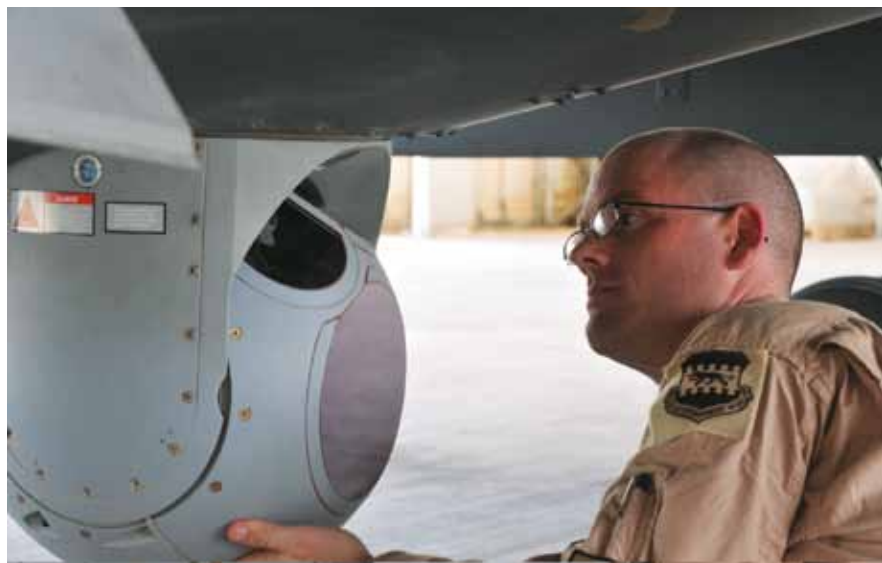
USAF SSgt. Aaron Pickering checks over the forward-looking infrared (FLIR) ball on an MC-12 Liberty before a mission at Joint Base Balad in Iraq. The first Liberty aircraft arrived in Iraq in June 2009.
