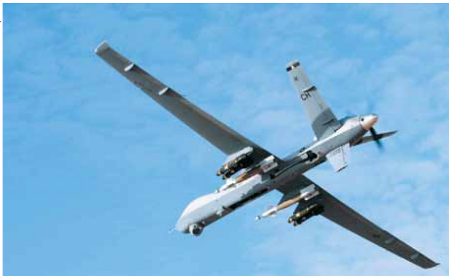
The Predator's big brother, the MQ-9 Reaper carries four Hellfires and two GBU-12 laser guided bombs.
