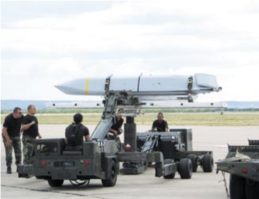
Airmen at Dyess AFB, Tex., ready a Joint Air-to-Surface Standoff Missile (JASSM) to be loaded onto a B-1B.
