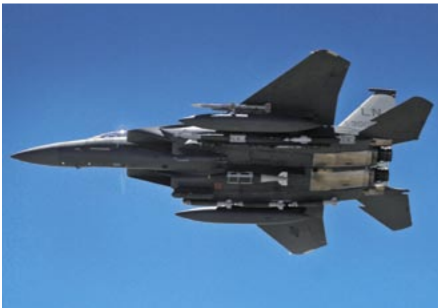
This USAF F-15E, over Afghanistan, bristles with weaponry—a JDAM, laser guided bombs, and an AIM-120 Advanced Medium-Range Air-to-Air Missile.
