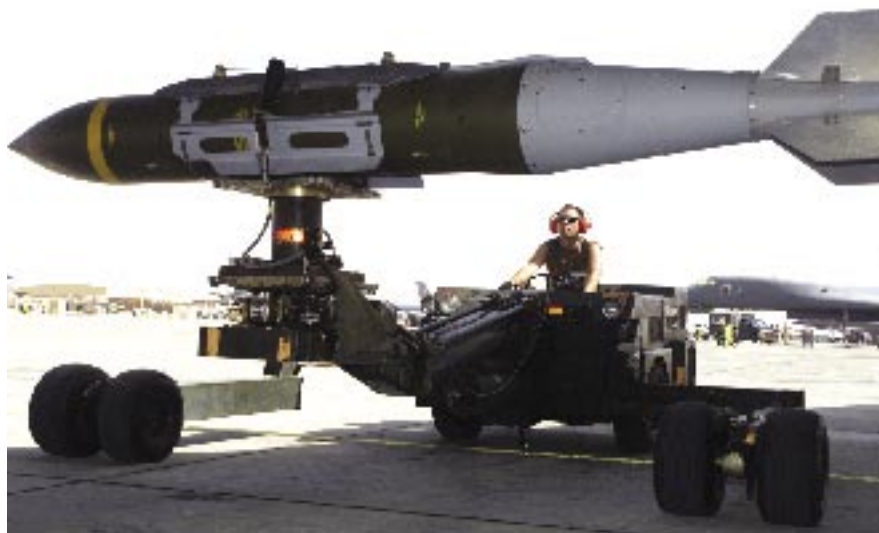
The GBU-31 JDAM consists of a bomb body, taken from inventory, a tail kit guidance section, and a set of strakes that help it maintain a precise aim angle. The near-precision weapon has changed the calculus of air attack.
