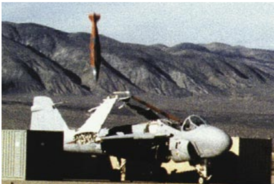
This is a test JDAM about to ruin the hulk of an A-6 Intruder. JDAM operates by inertial measurement, coupled with updates from the Global Positioning System. The result is a bomb that routinely hits within 10 feet of the aim point.
