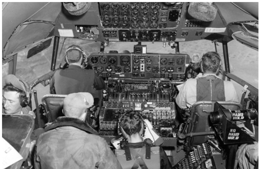
The XC-99's ample cockpit accommodated a sizeable crew. When the airplane was in service, USAF noted that the pilot and flight engineer were responsible for overseeing more than 250 gauges, switches, and levers.
