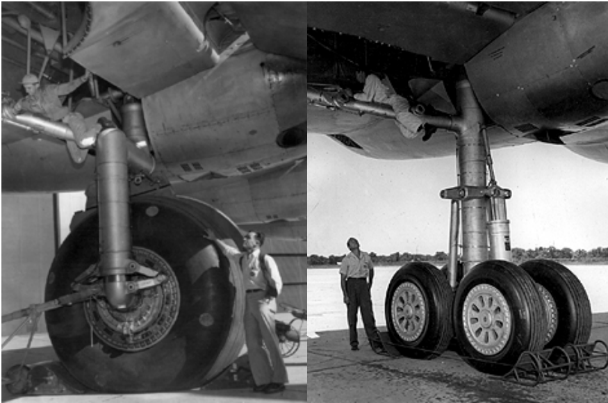
The image at left shows one of the two huge tires initially used for XC-99 landing gear. The image at right shows one set of the four-wheel system—used on production B-36s—that was retrofitted to the XC-99.
