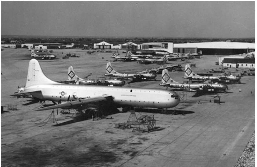
The XC-99, shown on a flight line alongside B-50s—the Air Force's workhorse bomber of the time—was derived from the B-36, but it was 20 feet longer, with a tail 10 feet taller. XC-99 dwarfed its contemporary aircraft.
