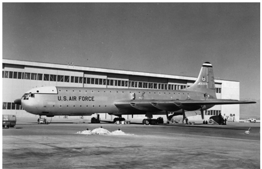
USAF took formal delivery of the XC-99 in 1949 and flew the aircraft until 1957. Early in its brief tenure, the XC-99 received its upgraded landing configuration and a nose radar unit.
