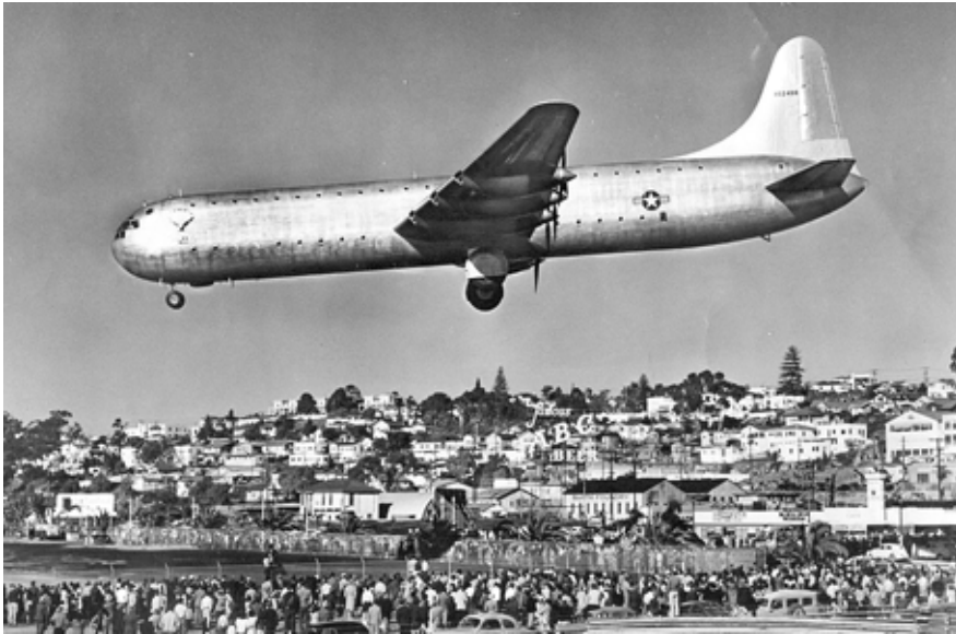
The XC-99 comes in for a landing during its November 1947 maiden flight out of Lindbergh Field, Calif. It was, at the time, the world's largest land aircraft. The transport required a 3,000-foot runway to take off and a 5,000-foot runway to land.
