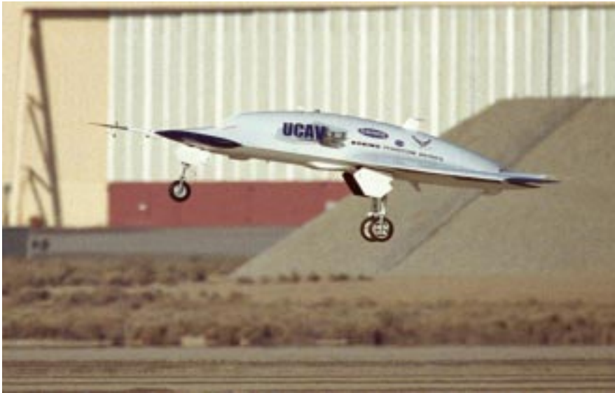
The UCAV flares for landing, after a 14-minute first flight. Handling qualities were judged to be good, and the no-tail airplane was stable throughout the flight. Testing will focus on mission, rather than violent maneuvering.
