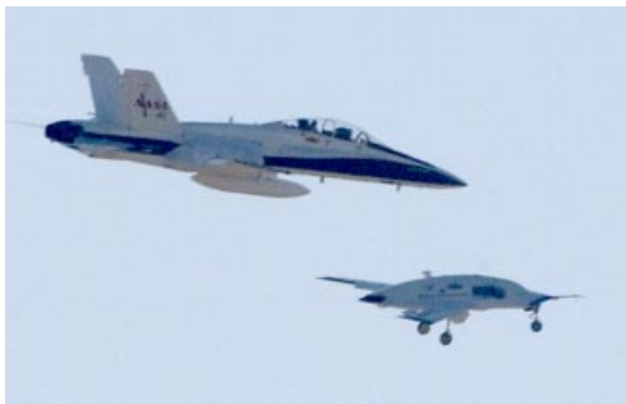
Gear was not retracted on the first flight, which is typical for a prototype. In combat, UCAVs may fly formation with manned aircraft, peeling off to strike pop-up air defense threats, or on their own, flying pre-emptive SEAD.
