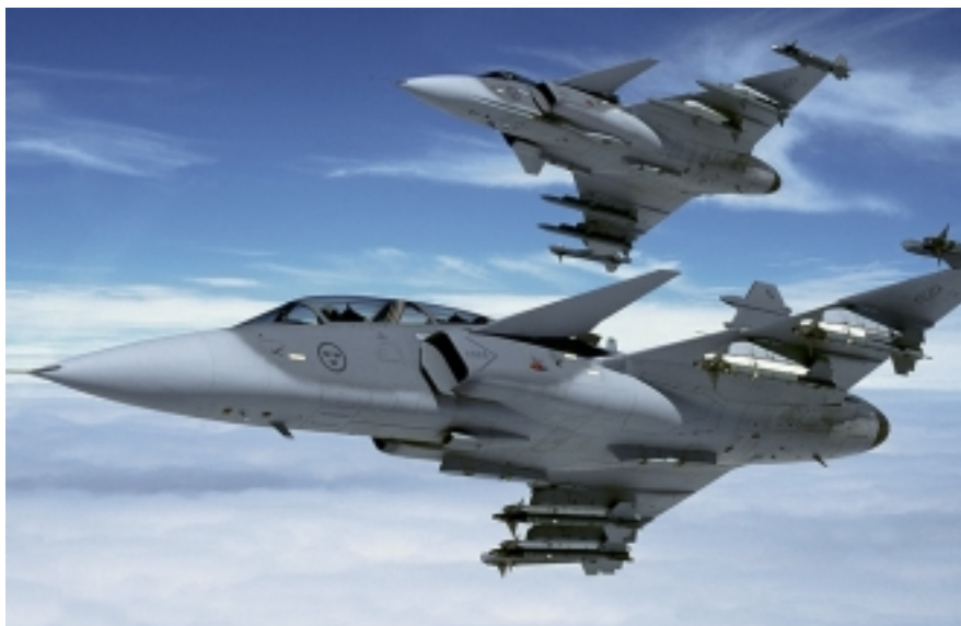
The JAS-39 Gripen is Sweden's 21st century fighter. Small and agile, it's easy to fix in the field, has advanced avionics, some stealth, and multirole capability. South Africa will be the first export customer.
