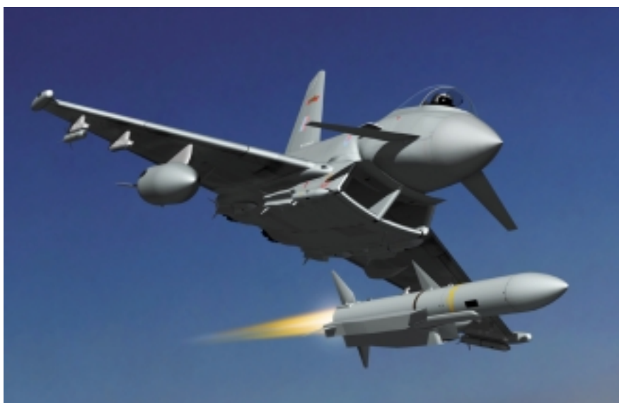
New, superfast, and extremely agile missiles pose an increased threat. The already potent Typhoon will give up its AMRAAMs for the Meteor, a ramjet-powered, long-range missile with high speed and resistance to countermeasures.
