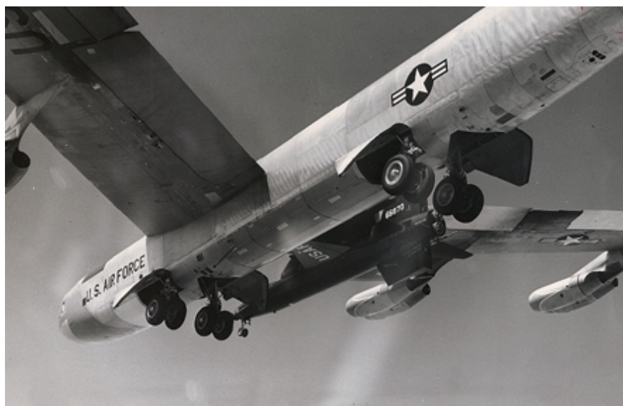
Only three A model B-52s were produced. One—designated NB-52A—served as the mother ship for the X-15 research aircraft and other test vehicles until 1968. After that a B model—NB-52B—took over.
