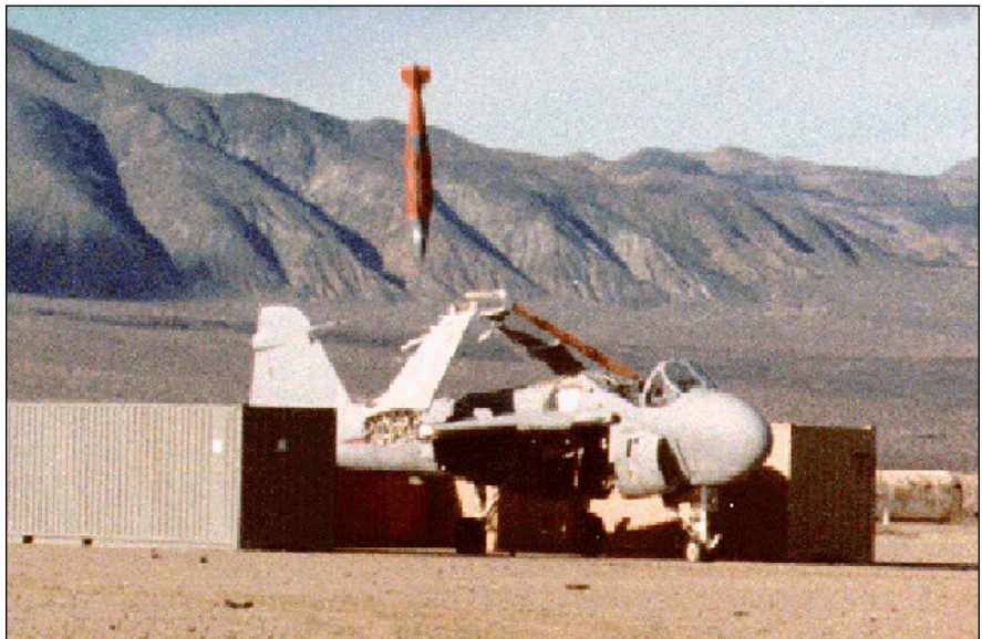
JDAM was the star performer of Allied Force and vindicated USAF's move to GPS-aided weapons. Seen here in a test against an A-6 carcass, JDAM is classed as a near-precision weapon but routinely hits within 40 feet of its target.
