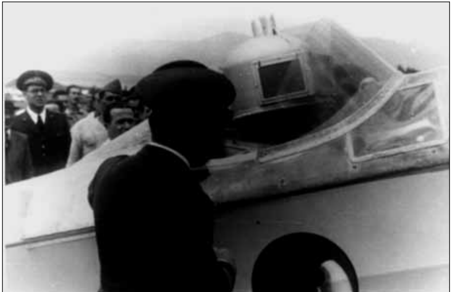
The Europeans set several altitude records in the 1930s, two of them in a Caproni 161 flown by Lt. Col. Mario Pezzi, who reached more than 50,000 feet. In both photos, Pezzi wears an aluminum pressure helmet with electrically heated glass ports.
