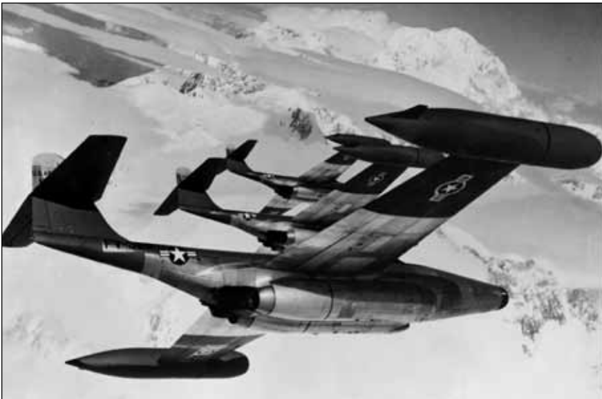
These three F-89D Scorpions, assigned to the 64th Fighter-Interceptor Squadron, Elmendorf AFB, Alaska, performed air defense duty in the Arctic, from Alaska to Greenland and Iceland. This model carried 104 2.75-inch folding-wing air-to-air rockets in its wingtip pods.
