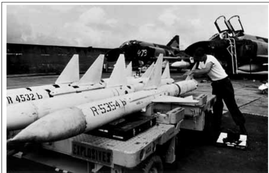
The F-4 carried four close-range AIM-9 Sidewinder heat-seeking missiles and four radar-guided AIM-7 Sparrows like those shown here. In the opening moments of Operation Bolo combat, Olds scored his first MiG-21 kill with an AIM-9.
