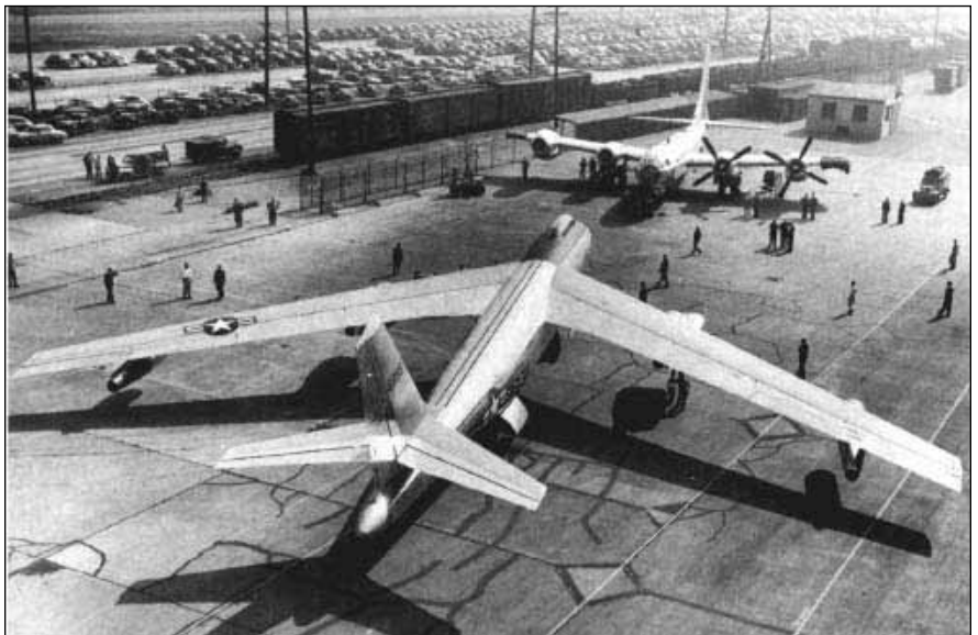
The future unveiled. In this early press release photo, Boeing's "radical" XB-47 Stratojet faces a partially completed B-50, the last propeller-driven bomber delivered to the Air Force.
