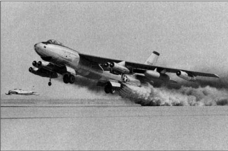
Any B-47 takeoff was interesting, but when ATO bottles were used, it was spectacular. Early B-47s had 18 bottles mounted internally. Later versions had an external 33-bottle unit.
