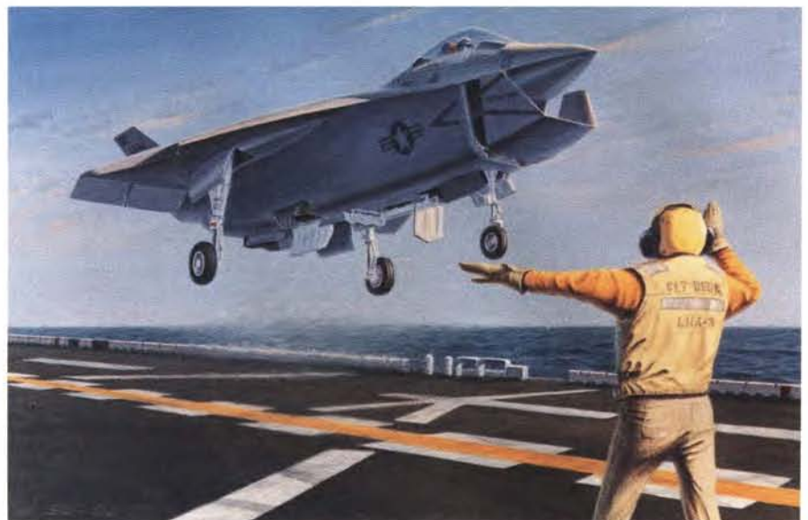
Boeing’s entry features an expandable inlet to gulp air for short takeoff and vertical landing operations. All JSF entries will be STOVL-capable, possibly paving the way toward smaller Navy carriers.
