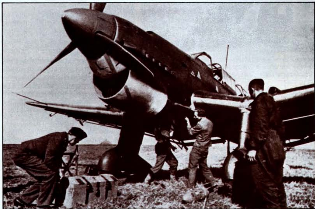
Here, Germans service a Ju-87 during the early days of the war. Despite its shortcomings, the Stuka was able to plunge toward its earthbound targets at speeds often in excess of 350 mph. (Photo courtesy of the United States Air Force Museum)
