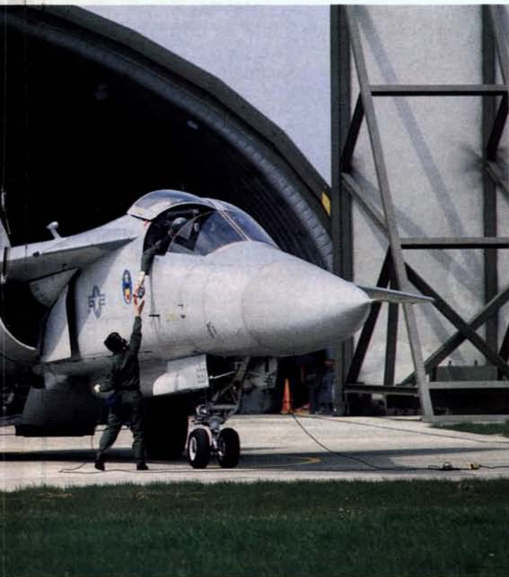
Even though it is unarmed, the Grumman EF-111A Raven is one of the most potent aircraft in the Air Force's inventory because of its ability to jam enemy electronic defenses. The Air Force has forty-two EF-111s divided between the 366th TFW at Mountain Home AFB, Idaho, and the unit this Raven belongs to, the 20th TFW at RAF Upper Heyford in the United Kingdom. (Photo © Mi Seitelman/IDI)
