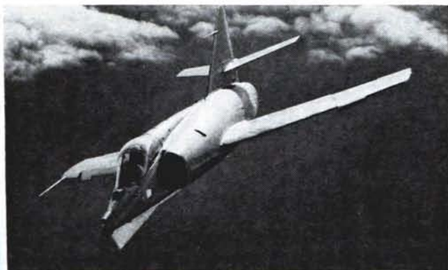
Another member of the French Air Force is the Etendard IV, also built by Dassault. It is a single-seat supersonic interceptor and ground-support aircraft built originally to French AF requirements but ordered instead by the Navy for service aboard new French aircraft carriers.
