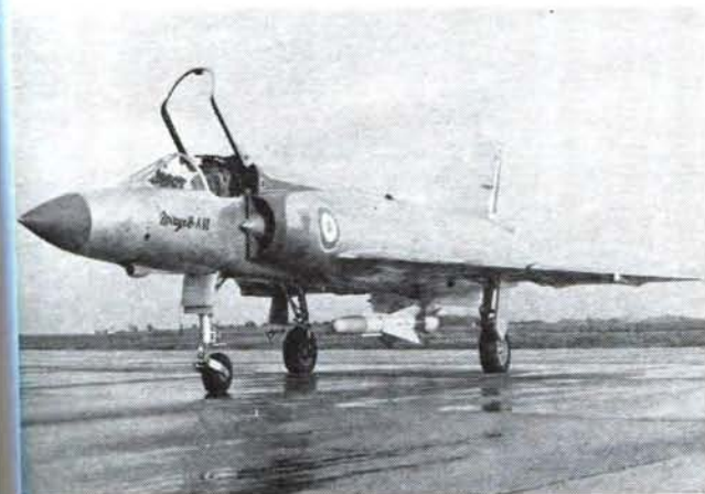
The Mirage IIIA, strikingly similar to the Mirage IV strategic bomber, is a single-seat supersonic fighter designed for high-altitude interception as well as tactical, all-weather support. Like the Mirage IV, it flies at Mach 2.
