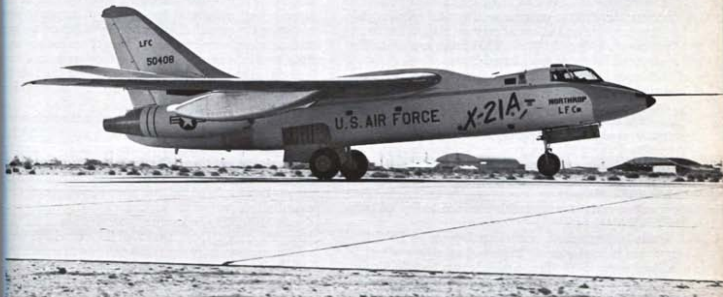
USAF/Northrop X-21 Laminar Flow Control aircraft lands at Edwards AFB, Calif., after a flight test of its air-inhaling wings. Although it is still early in the flight-test program, the X-21 has demonstrated substantial reduction of friction drag.
