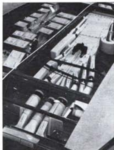
Shown in the mockup at right is the elaborate system of ducts that connects the X-21's pumping system to long ducts built into the wings. Valves control the suction system's pressures. The operational system would be more simple.
