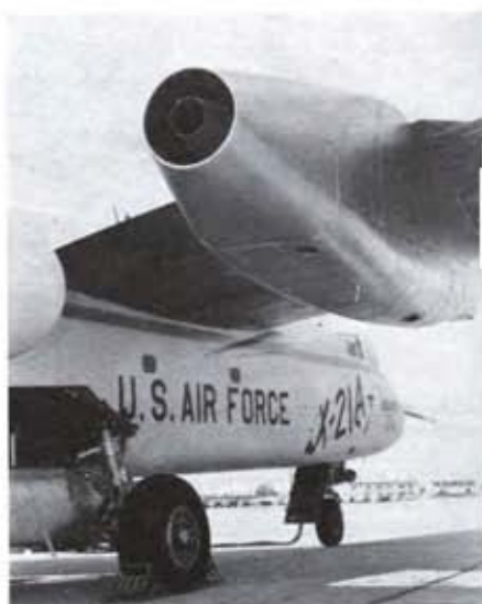
Space problems on X-21 experimental aircraft are emphasized in photo at right, showing aft end of wing-mounted LFC pumping system (on right side) and J79 inlet (left side). Operational LFC aircraft would have a more simplified arrangement.
