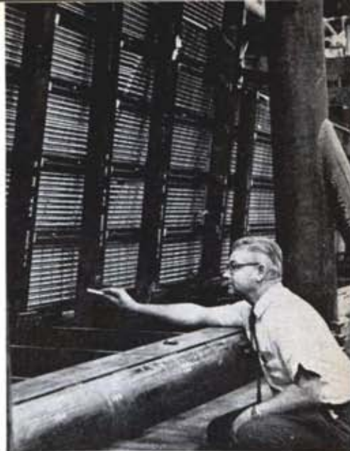
X-21 wing in production jig shows rows of tributary ducts bonded in place. Tributary ducts are needed to maintain nearly constant pressures in wing ducts, thus preventing high flow losses.
