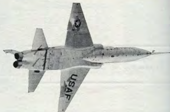
Underbelly view shows T-38 design features including the contoured fuselage, flat afterbody, split between engines.
