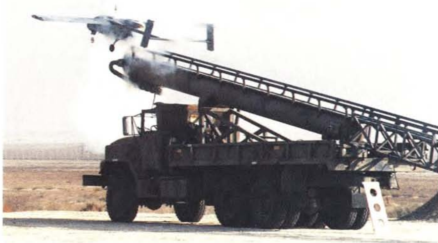
The Pioneer needs no airstrip, and it has seen extensive use already, including reconnaissance missions over the Persian Gulf, Haiti, Somalia, and Bosnia-Herzegovina. It has an action radius of 115 miles and can stay aloft for five hours.
