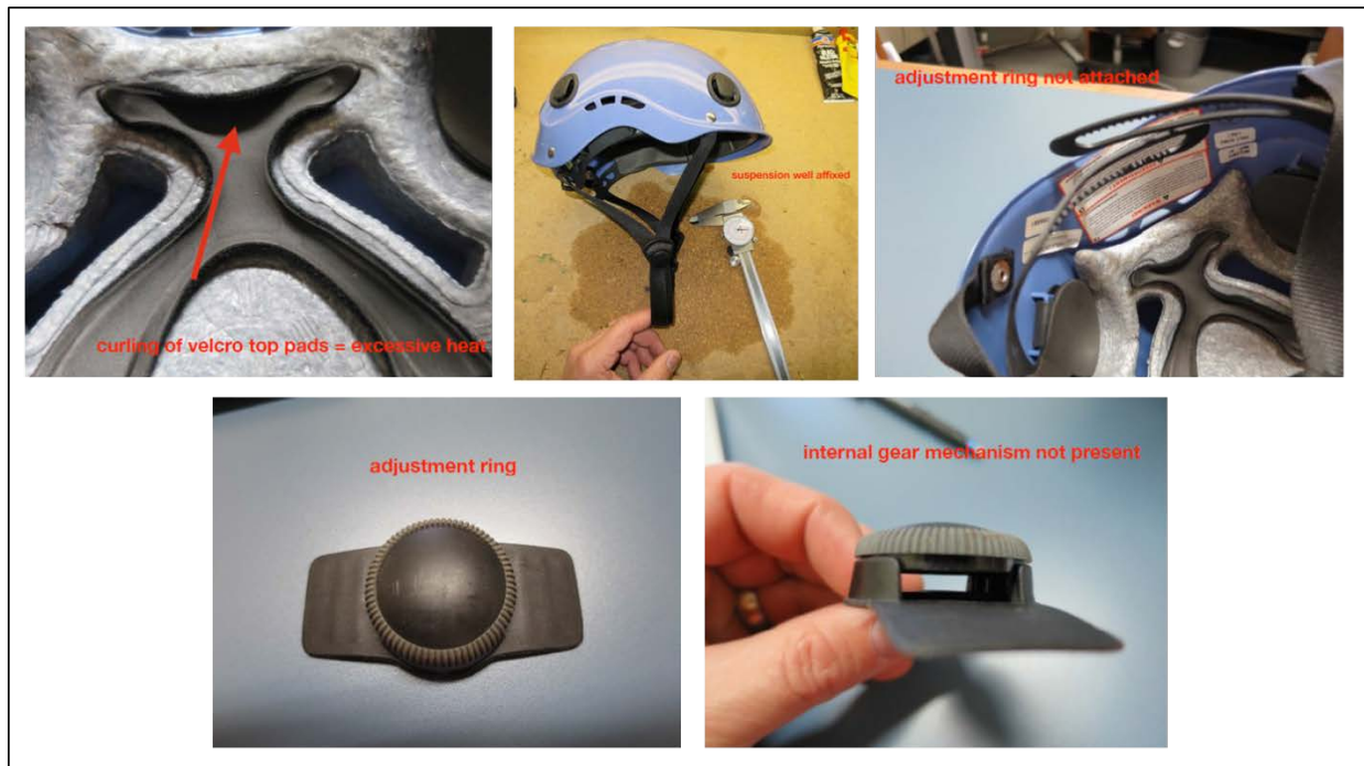
Figure 22: Visual inspection and comparative baseline analysis of the internal suspension harness on mishap helmet (Tab CC-36 thru CC-37)
