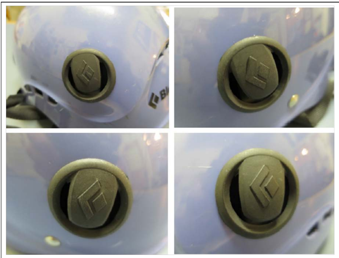
Figure 28: Headlamp inspection and comparison to baseline on mishap helmet (Tab CC-43 thru CC-44)
