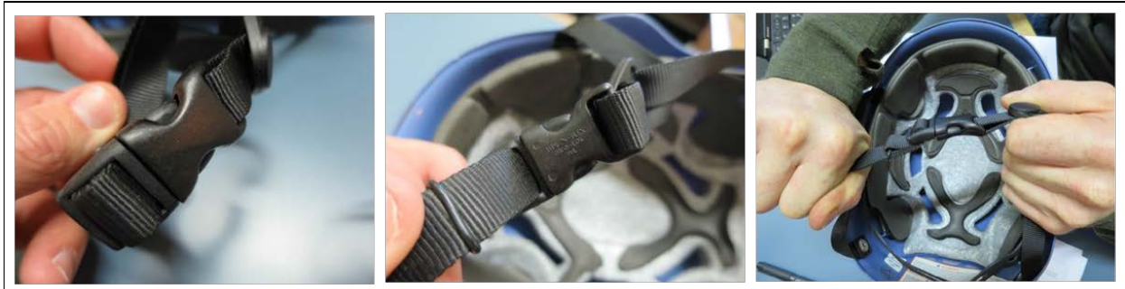
Figure 23: Visual inspection of the chin strap buckle on mishap helmet (Tab CC-38)
