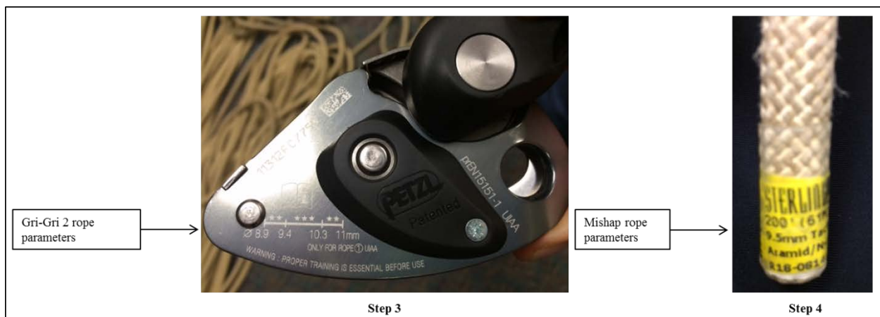
Figure 16: Petzl Gri-Gri 2 evaluation steps 3-4 (Tabs CC-4, CC-8)
