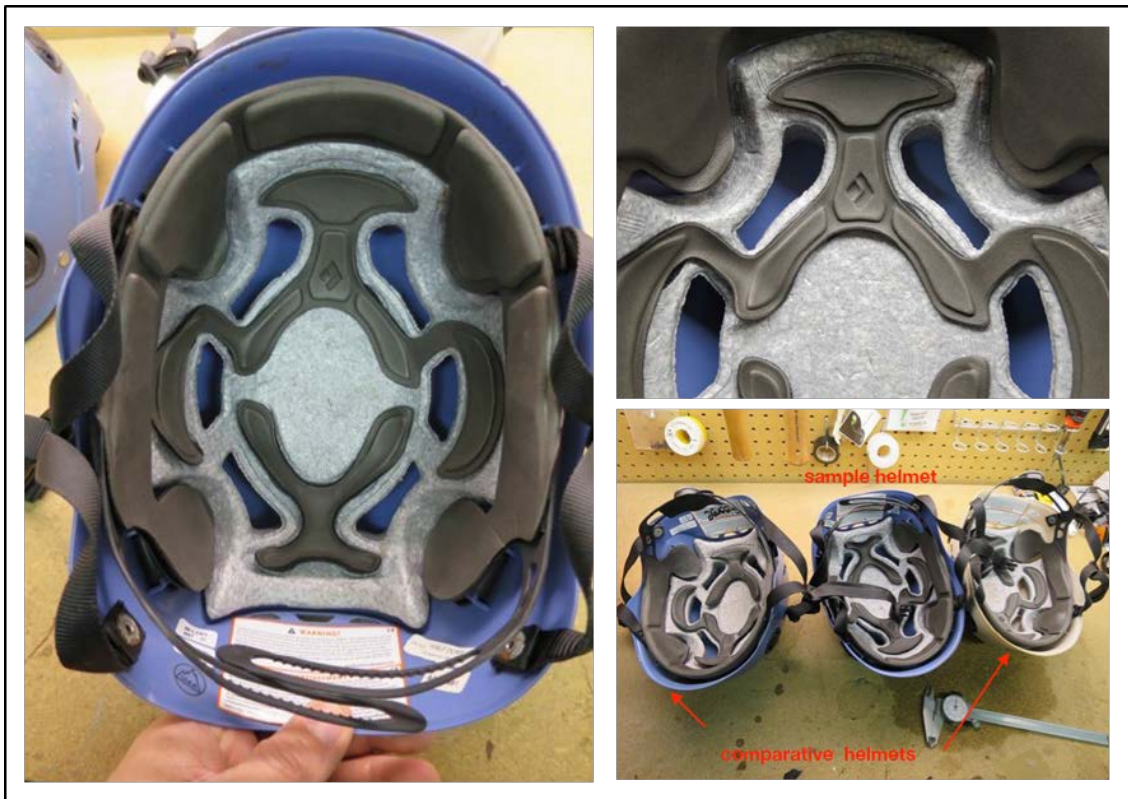
Figure 24: Visual inspection and dimensional inspection of the EPS liner on mishap helmet (Tab CC-39)
