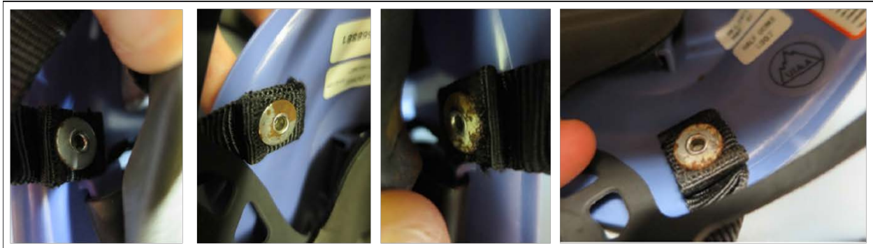
Figure 27: Rivet inspection and comparison to baseline on mishap helmet (Tab CC-43)
