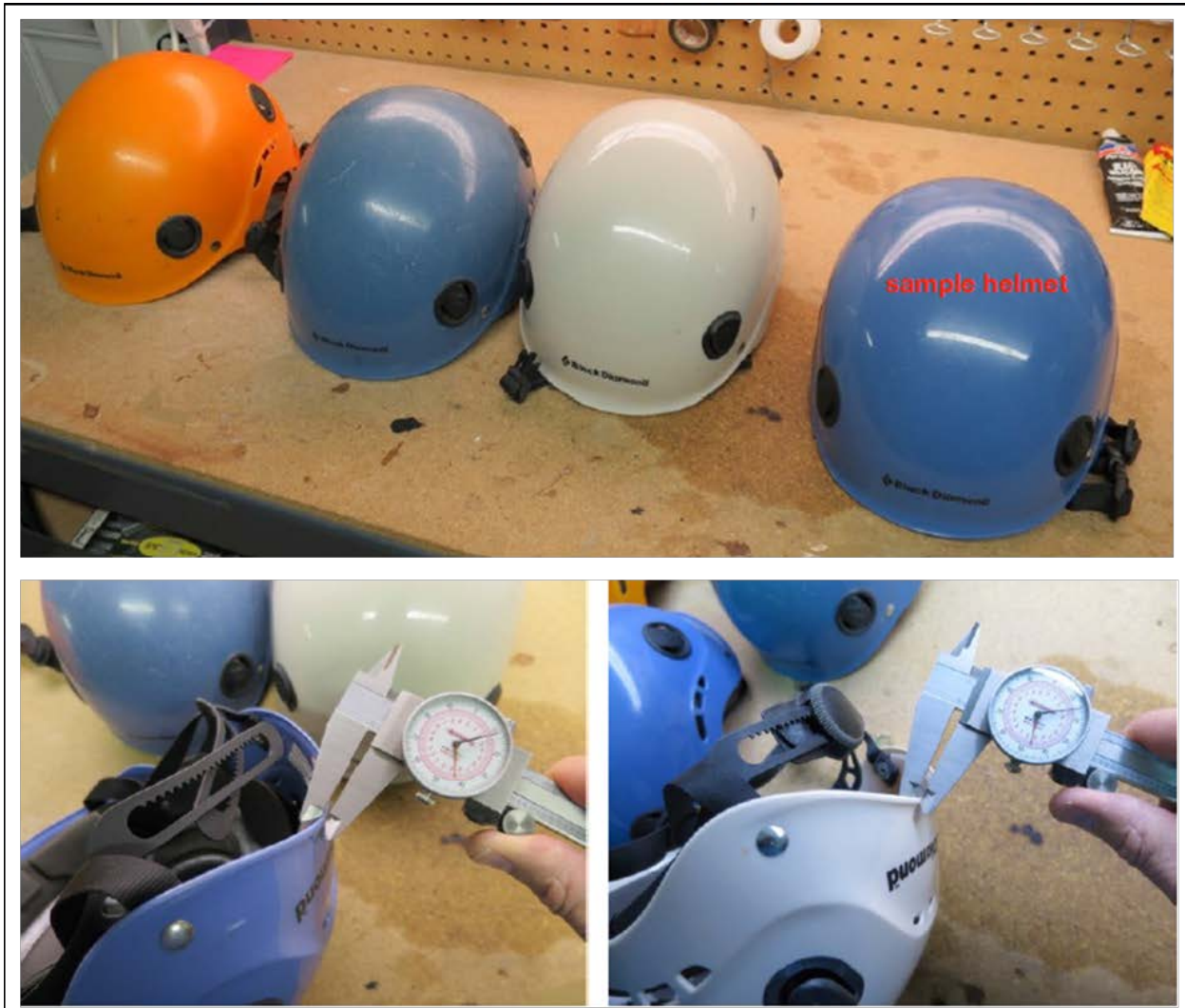
Figure 26: Visual inspection and dimensional inspection of the ABS shell on mishap helmet (Tabs CC-40, CC-42)
